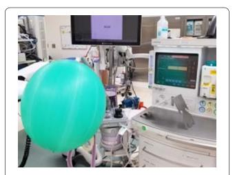
**Figure 16.** Anesthesia machine inadvertently left in test mode with high flow and 20 mm Hg pressure on pop-off valve.
